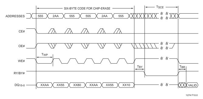
Note: This device also supports CE# controlled Chip-Erase operation. The WE# and CE# signals are interchageable as long as minimum timings are met. (See Table 14) X can be VIL or VIH, but no other value.
