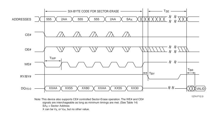
FIGURE 14: WE# CONTROLLED SECTOR-ERASE TIMING DIAGRAM
