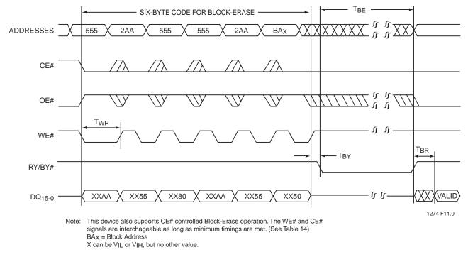
FIGURE 13: WE# CONTROLLED BLOCK-ERASE TIMING DIAGRAM
