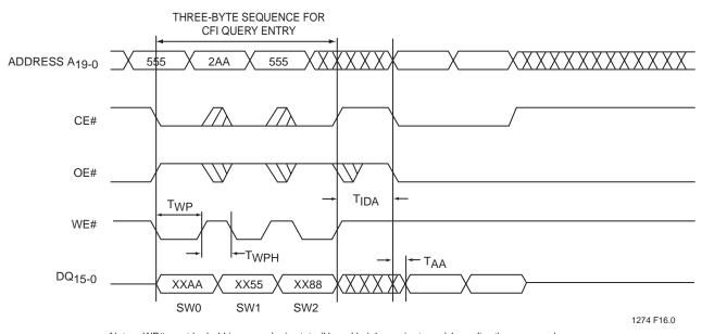
Note: WP# must be held in proper logic state (V<sub>IL</sub> or V<sub>IH</sub>) 1  $\mu$ s prior to and 1  $\mu$ s after the command sequence X can be V<sub>IL</sub> or V<sub>IH</sub>, but no other value.
