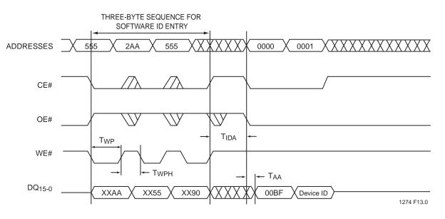
Device ID = 734BH for SST36VF1601E and 734AH for SST36VF1602E Note: X can be  $V_{IL}$  or  $V_{IH},$  but no other value.
