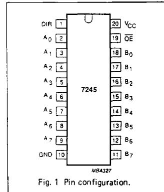
Fig. 1 Pin configuration.
