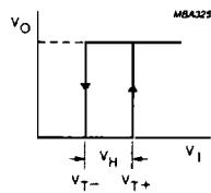
Fig. 4 Transfer characteristic.
