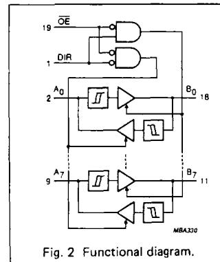
Fig. 2 Functional diagram.
