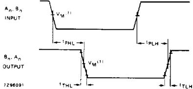
Fig. 6 Waveforms showing the input ( $A_n, B_n$ ) to output ( $B_n, A_n$ ) propagation delays and the output transition times.
