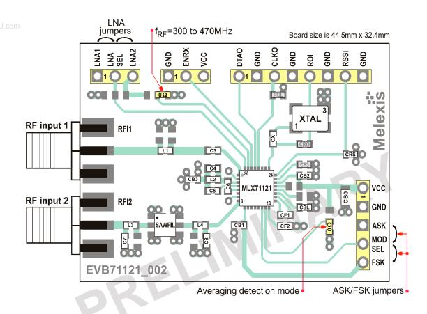
Fig. 6: PCB top-side view
