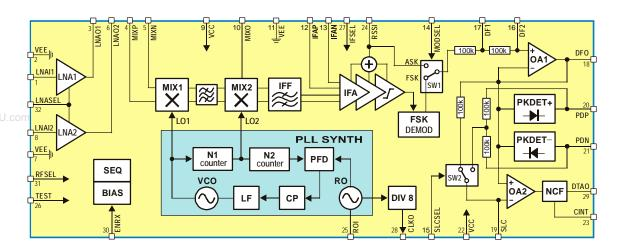
Fig. 1: MLX71121 block diagram
