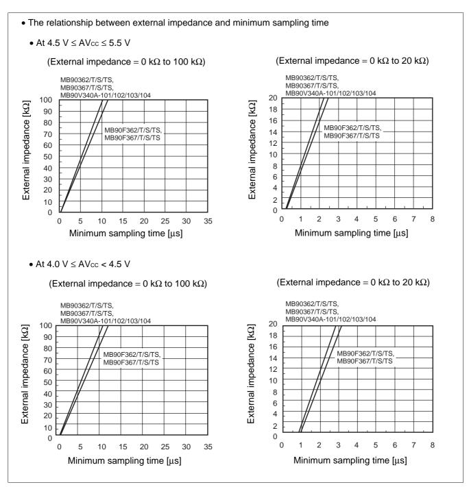
If the sampling time cannot be sufficient, connect a capacitor of about 0.1 μF to the analog input pin.
