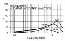
Test equipment L, Q: YHP4194A IMPEDANCE ANALYZER (16085A+16093B+TDK TF-1)
