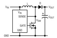
2a. SENSE Pin Connection for Maximum Efficiency (V<sub>SW</sub> < 36V)
