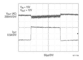
Figure 19. LTC1871-1 SEPIC Converter Load Step Response
