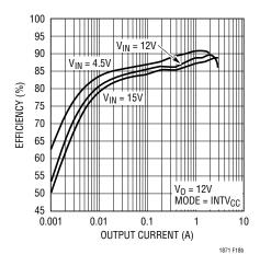
Figure 18b. SEPIC Efficiency vs Output Current
