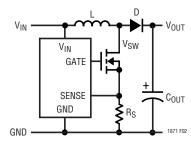
2b. SENSE Pin Connection for Precise Control of Peak Current or for V<sub>SW</sub> > 36V
