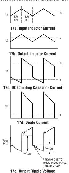
Figures 17. SEPIC Converter Switching Waveforms
