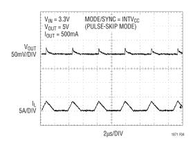
Figure 4. LTC1871-1 Low Output Current Operation with Burst Mode Operation Disabled (MODE/SYNC = INTV<sub>CC</sub>)
