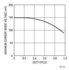
Figure 10. Maximum SENSE Threshold Voltage vs Duty Cycle
