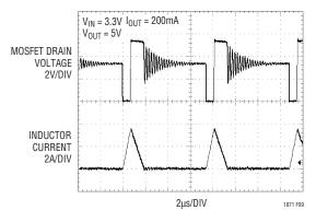
Figure 9. Discontinuous Mode Waveforms
