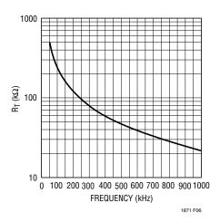
Figure 6. Timing Resistor (R<sub>T</sub>) Value
