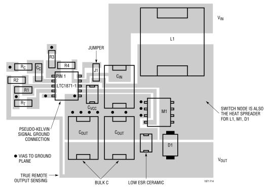
Figure 14. LTC1871-1 Boost Converter Suggested Layout
