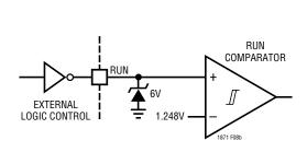
Figure 8b. On/Off Control Using External Logic
