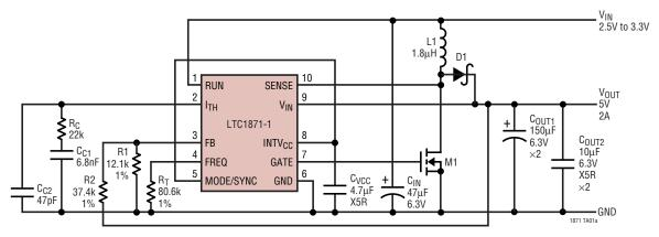
C<sub>IN</sub>: SANYO POSCAP 6TPA47M C<sub>OUT1</sub>: SANYO POSCAP 6TPB150M C<sub>OUT2</sub>: TAIYO YUDEN JMK316BJ106ML C<sub>VCC</sub>: TAIYO YUDEN LMK316BJ475ML
