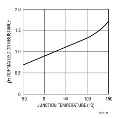
Figure 11. Normalized R<sub>DS(ON)</sub> vs Temperature
