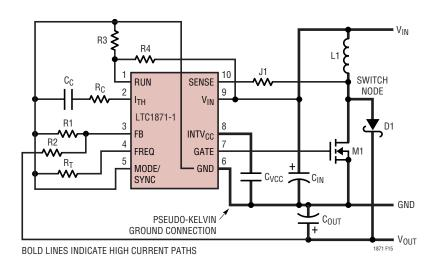
Figure 15. LTC1871-1 Boost Converter Layout Diagram
