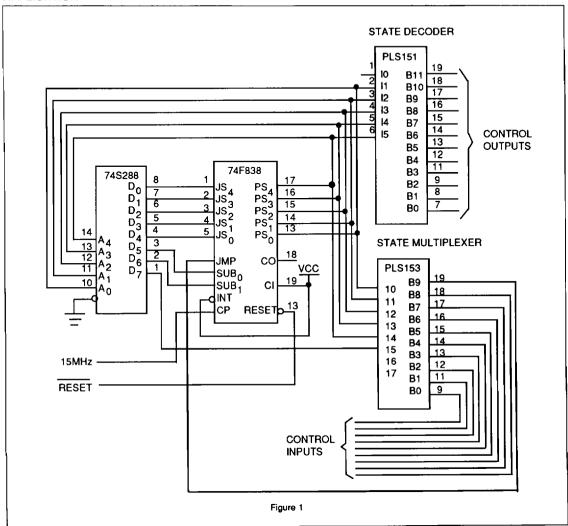
As shown in Figure 1, a PROM paired with a 74F838 creates a state machine. When reset, the PS<sub>0</sub>-PS<sub>4</sub> outputs are zero. The present state is decoded to generate control inputs. In this application, a PLS151 acts as the state decoder. When a state has a branch option
