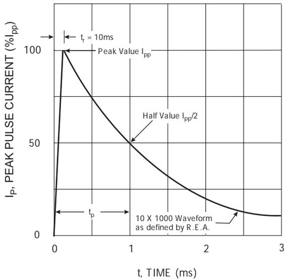
Fig. 1 Pulse Waveform
