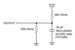
Figure 1: AC Output Loading
