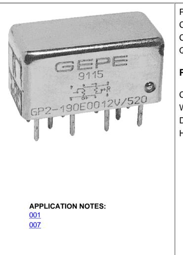
Polarized, latching hermetically sealed relayContact arrangement2 PDTCoil supplyDirect currentQualified toSCC3602/003
