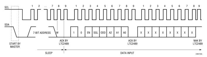
Figure 3b. Timing Diagram for Writing to the LTC2489
