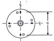
A = OUTSIDE DIAMETER B = HEIGHT C = CORE DIAMETER D = LEAD SPACING
