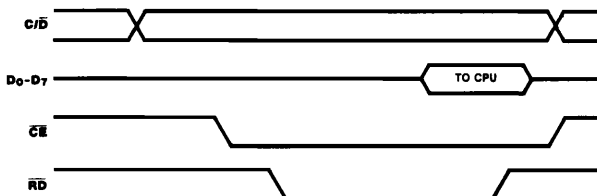
Figure 9. Non-Z-BUS Read Cycle Timing
