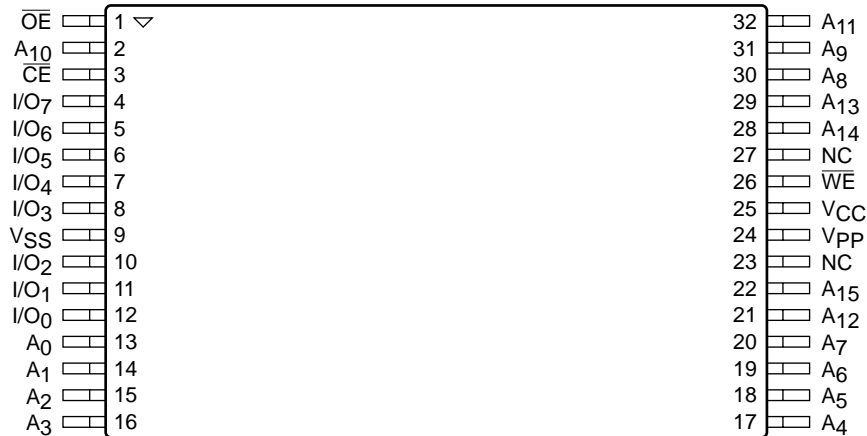
TSOP Package (Reverse Pinout) (TR, HR)
