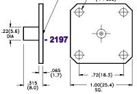
Note: All Models are available with EMI gasketed flange face, designate by subsituting "EMI" for "FLG" in Model No.
