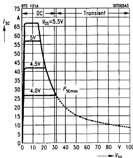
**Max. gate voltage  $V_{GS(SC)} = f(V_{DS})$** Parameter:  $T_j = -55 \dots +150^\circ\text{C}$
