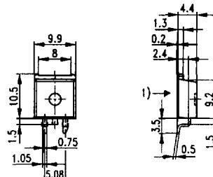
1) shear and punch direction no burrs this surface
