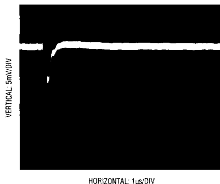
Figure 11. Adequate Settling of Op Amp Driving Analog Input
