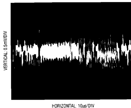
Figure 7. Poor V_{CC} Bypassing. Noise and Ripple can Cause A/D Errors
