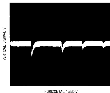
Figure 15. Adequate Reference Settling
