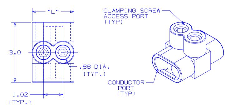
TWO PORT CONNECTOR BLOCK SHOWN WITH PLASTIC CLOSURE PLUGS REMOVED. SEE TABLE FOR DIMENSIONS OF PARTS WITH ADDITIONAL PORTS.
