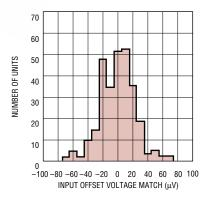
$V_S = \pm 15V$   $T_A = 25^{\circ}C$ 287 LINITS TESTED
