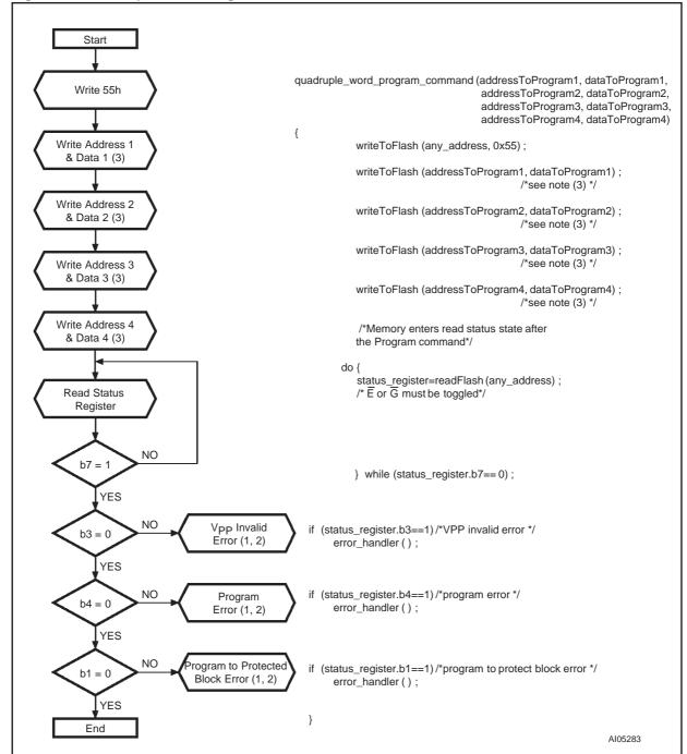
Figure 20. Quadruple Word Program Flowchart and Pseudo Code
