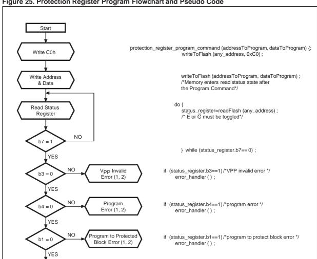
Figure 25. Protection Register Program Flowchart and Pseudo Code
