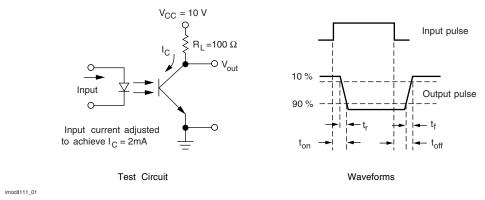
Fig. 1 - Switching Times
