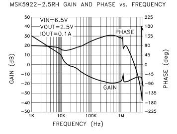
MSK5922-2.5RH GAIN AND PHASE vs. FREQUENCY
