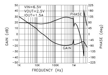
MSK5922-2.5RH GAIN AND PHASE vs. FREQUENCY
