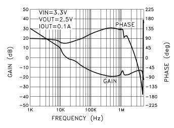
MSK5922-2.5RH GAIN AND PHASE vs. FREQUENCY
