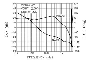
MSK5922-2.5RH GAIN AND PHASE vs. FREQUENCY
