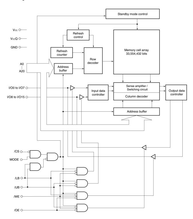
$\textbf{Remark}\ \ \mathsf{Vcc} Q$  is the input / output power supply for -BE75X and -BE85X.
