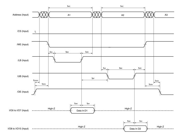
Figure 6-11. Write Cycle Timing Chart 5 (/LB, /UB Independent Controlled)
