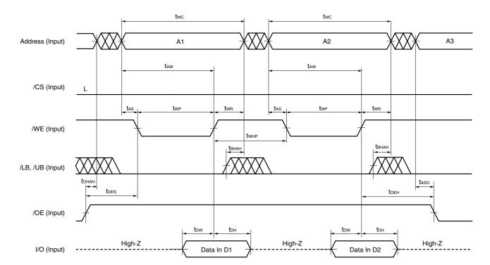
Figure 6-9. Write Cycle Timing Chart 3 (/WE Controlled)
