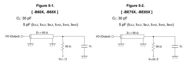
Remark CL includes capacitance of the probe and jig, and stray capacitance.
