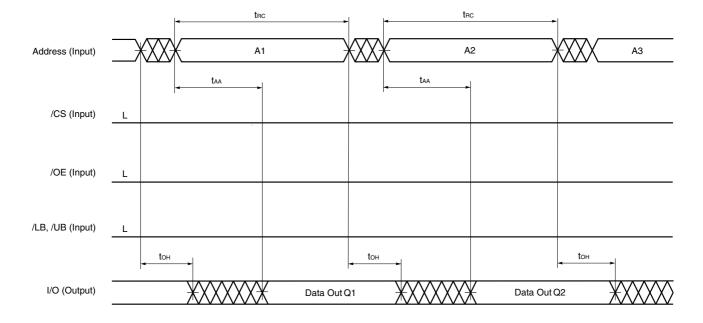
Figure 6-4. Read Cycle Timing Chart 4 (Address Controlled)
