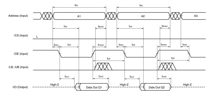
Figure 6-2. Read Cycle Timing Chart 2 (/OE Controlled)
