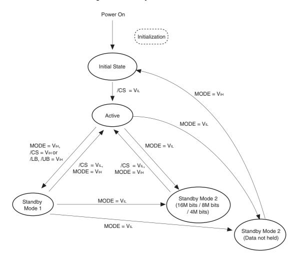
Figure 2-1. Standby Mode State Machine
