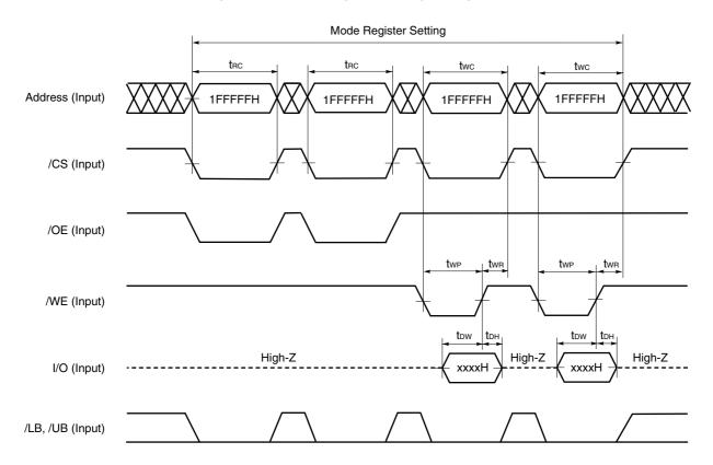
Figure 6-12. Mode Register Setting Timing Chart
