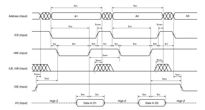
Figure 6-8. Write Cycle Timing Chart 2 (/WE Controlled)
