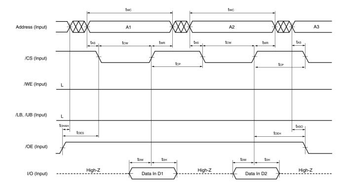
Figure 6-7. Write Cycle Timing Chart 1 (/CS Controlled)
