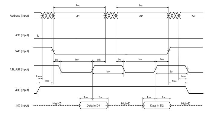
Figure 6-10. Write Cycle Timing Chart 4 (/LB, /UB Controlled)
