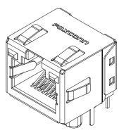
Mating Force: 4 Pounds Max. Unmating Force: 4 Pounds Max. Durability: 1000 Cycles Electrical Current Rating: 1.5A Max. Voltage Rating: 150 VAC Dielectric Withstanding Voltage: 1000V Contact To Contact 1500V Contact To Shield
