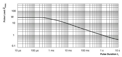
Maximum pulse load, single pulse; applicable if  $\bar{P} \rightarrow 0$  and n  $\leq 1000$  and  $\hat{U} \leq \hat{U}_{max}$ ; Single Pulse for permissible resistance change equivalent to 8000 h operation
