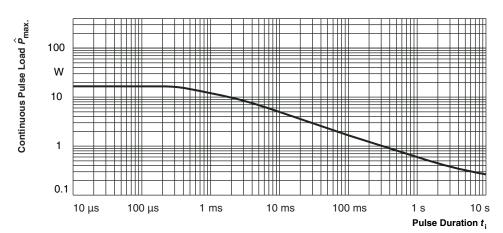
Maximum pulse load, continuous pulses; applicable if  $\bar{P} \leq P$  ( $\vartheta_{amb}$ ) and  $\hat{U} \leq \hat{U}_{max}$ ; for permissible resistance change equivalent to 8000 h operation
