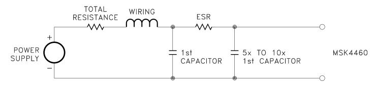
Be careful of the ripple current in all the capacitors. Excessive ripple current, beyond what the capacitors can handle, will destroy the capacitors.
