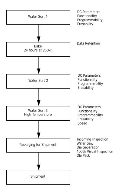
Figure I. Spansion KGD Product Test Flow
