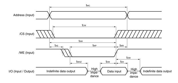
$\hbox{\it Cautions 1. /CS or /WE should be fixed to high level during address transition.}$
