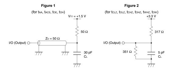
**Remark** C<sub>L</sub> includes capacitances of the probe and jig, and stray capacitances.
