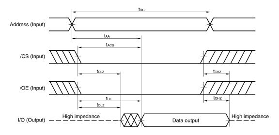
Caution Address valid prior to or coincident with /CS low level input.
