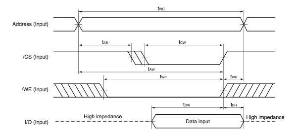
Cautions 1. /CS or /WE should be fixed to high level during address transition.
