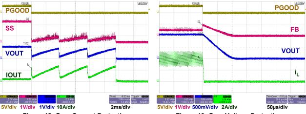
Figure 12: Over Current Protection (tested by shorting VOUT to PGND)
