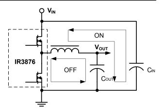
Figure 20. Current Path of Power Stage
