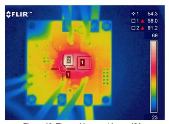
Figure 16: Thermal Image at I<sub>OUT</sub> = 12A (IR3876: 81°C, Inductor: 58°C, PCB: 54°C)
