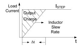
Figure 18. Charge Requirement during Load Step
