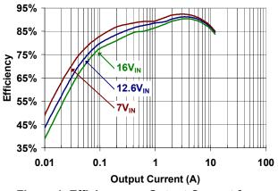
Figure 1. Efficiency vs. Output Current for VOUT = 1.05V, L = 1.2 $\mu$ H (2.9 $m\Omega$ )
