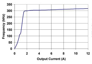
Figure 3. Switching Frequency vs. Output
