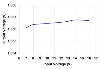
Figure 6. Output Voltage Regulation vs. Input Voltage at I<sub>OUT</sub> = 12A
