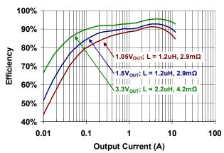
Figure 2. Efficiency vs. Output Current for VIN = 12.6V
