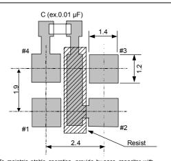
To maintain stable operation, provide by-pass capacitor with more than 0.1  $\mu\text{F}$  at a location as near as possible to the power source terminal of the crystal products (between VCC - GND).
