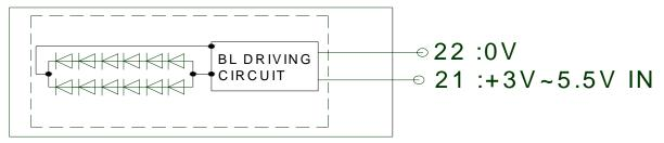
PIN22 is connected to PIN2(VSS) internally
