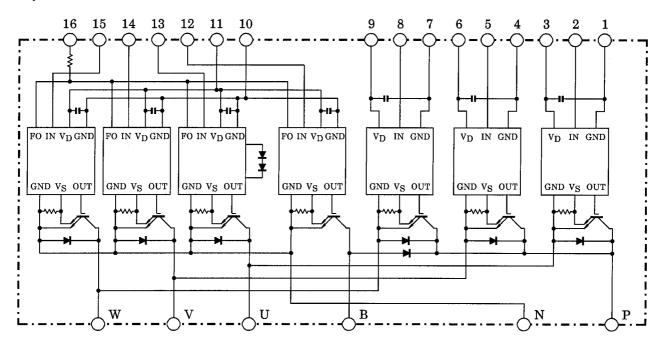
5. IN (V) 6.  $V_D(V)$ 1. GND (U) 2. IN (U) 3.  $V_D(U)$ 4. GND (V) 7. GND (W) 8. IN (W) 9.  $V_{\mathbf{D}}(W)$ 10.GND (L)  $11.V_{D}$  (L)  $12.\overline{IN}$  (B) 13.IN (X) 14.IN (Y) 15.IN (Z) 16.FO
