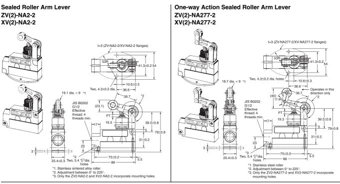
Note: Unless otherwise specified, a tolerance of  $\pm 0.4$  mm applies to all dimensions.
