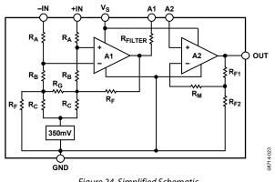
Figure 24. Simplified Schematic
