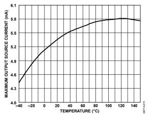
Figure 11. Maximum Output Source Current vs. Temperature
