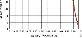
Figure 9. Input Bias Current of A2 vs. Input Voltage and Temperature
