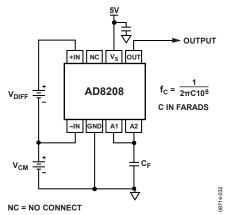
If the gain is raised using a resistor, as shown in Figure 31, the corner frequency is lowered by the same factor as the gain is raised. Therefore, using a resistor of 200 k $\Omega$  (for which the gain would be doubled), results in a corner frequency scaled to 0.796 Hz  $\mu F$  (0.039  $\mu F$  for a 20 Hz corner frequency).
