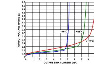
Figure 13. Output Voltage Range from GND vs. Output Sink Current
