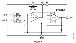
Automotive applications demand robust, precision components for improved system control. The AD8208 provides excellent ac and dc performance, minimizing errors in the application. Typical offset and gain drift in both the SOIC and MSOP packages are less than 5  $\mu$ V/°C and 10 ppm/°C, respectively. The device also delivers a minimum CMRR of 80 dB from dc to 10 kHz.
