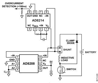
Figure 27. Battery-Referenced Shunt Resistor
