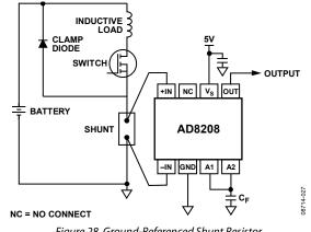
Figure 28. Ground-Referenced Shunt Resistor
