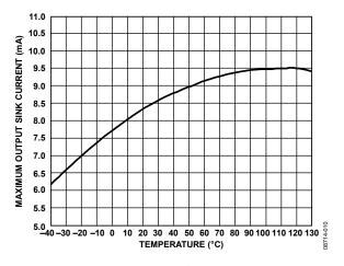
Figure 10. Maximum Output Sink Current vs. Temperature
