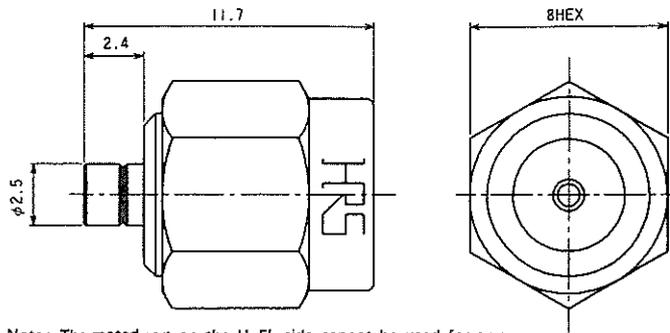
Note: The mated part on the H.FL side cannot be used for any purpose other than performance measurement because there is no lock mechanism.
