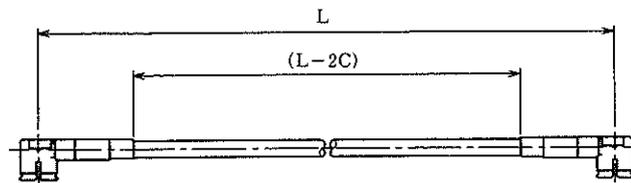
Specify the dimensions from the center of connectors for both single- and double-connector harnesses. Standard dimensional tolerances are as follows:
