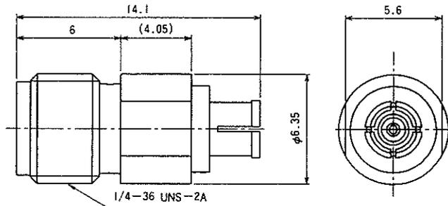
Note: The mated part on the H.FL side cannot be used for any purpose other than performance measurement because there is no lock mechanism.
