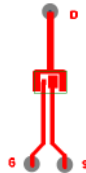
① Mounted on minimum footprint full size board with metalized back and with small clip heatsink (still air)
