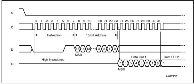
Figure 12. Read from Memory Array (READ) sequence
