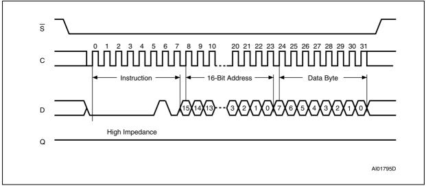
1. Depending on the memory size, as shown in Table 5, the most significant address bits are Don't Care.
