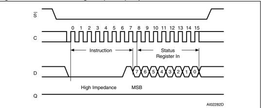
Figure 11. Write Status Register (WRSR) sequence
