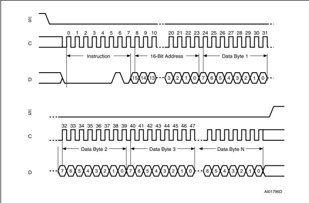
1. Depending on the memory size, as shown in *Table 5*, the most significant address bits are Don't Care.
