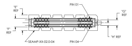
FIG. 3 -06: 6 ROWS (SAME AS FIG. 1, EXCEPT AS SHOWN) (SEAMP-20-02.0-X-06-TR SHOWN) (SOME CENTER FEATURES NOT SHOWN FOR CLARITY)
