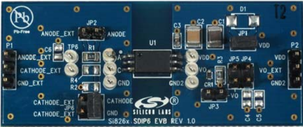
Figure 3. Si826x SDIP6 Evaluation Board Overview
