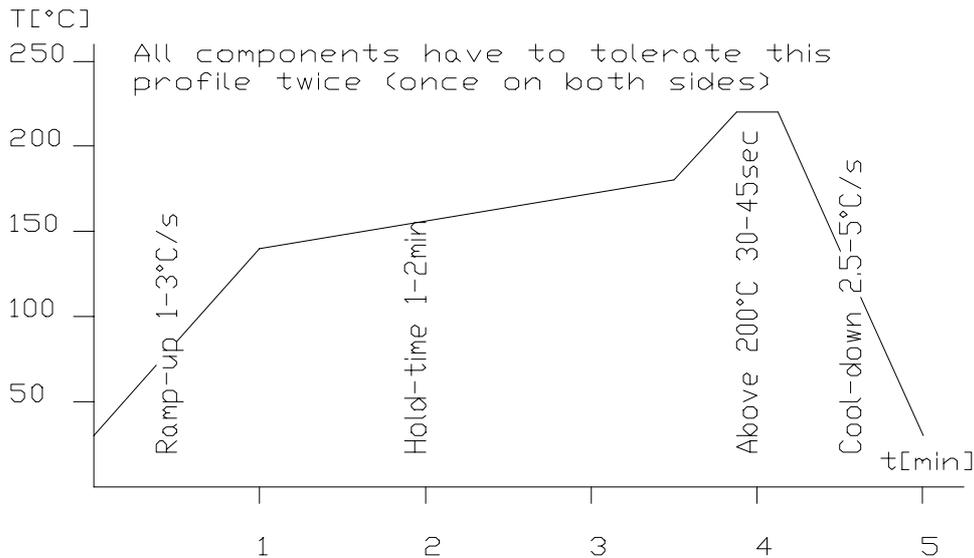
**Note :** Reflow profile to use depends on solder characteristics. Each soldering material supplier has its own recommendation. This profile is use for the product qualification step.
