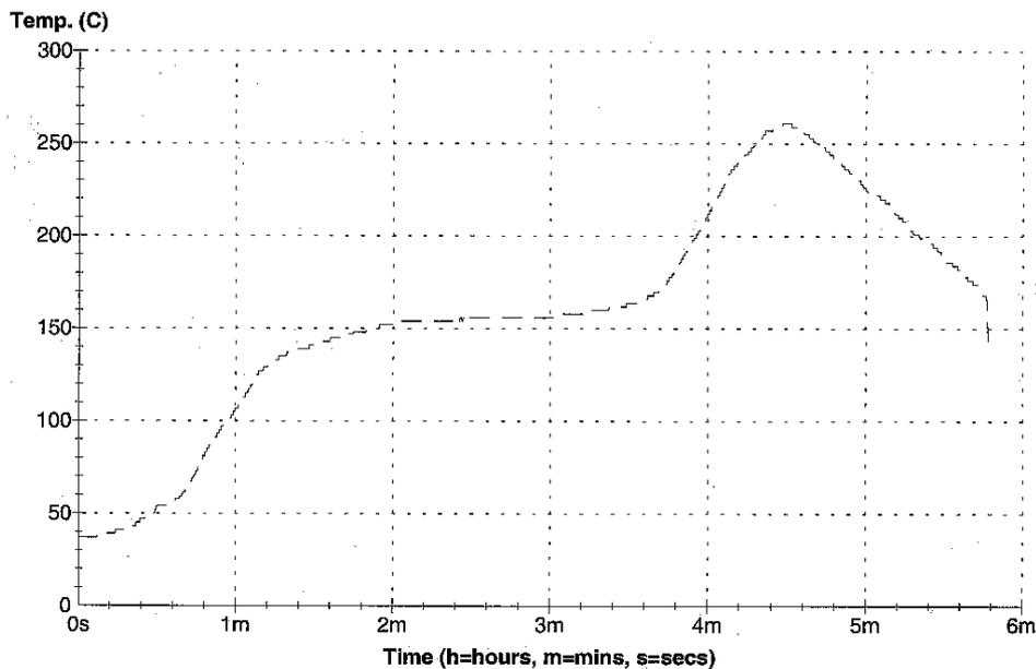
**Note :** Reflow profile to use depends on solder characteristics. Each soldering material supplier has its own recommendation. TEMEX use the above temperature profile to test reflow compliance of products. Usually the temperature peak is around 250-260 °C during 10 to 20 secondes.
