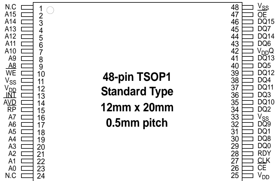
(TOP VIEW, Facing Down) TSOP1 OneNAND Chip 48pin, 12mm x 20mm, 0.5mm pitch TSOP1
