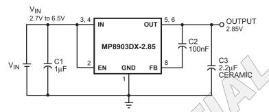
Figure 3—Typical Application Circuit (Fixed)
