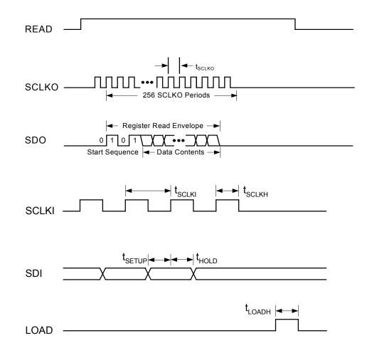
Figure 5. Output Phase Adjust Timing Diagrams (Register Control)
