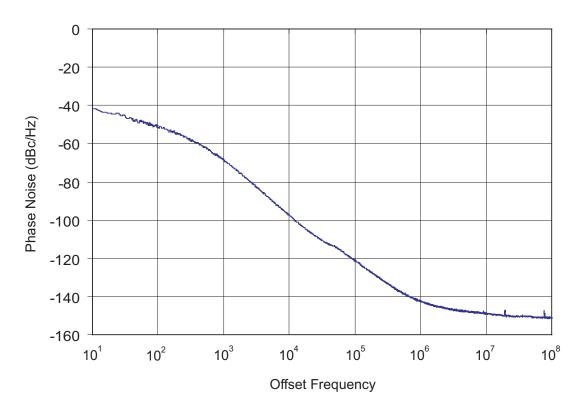
Figure 6. Typical Si5320 Phase Noise (CLKIN = 155.52 MHz, CLKOUT = 622.08 MHz, and Loop BW = 800 Hz)
