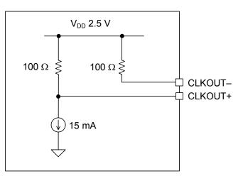
Figure 10. CLKOUT± Equivalent Circuit, RSTN/CAL Asserted LOW
