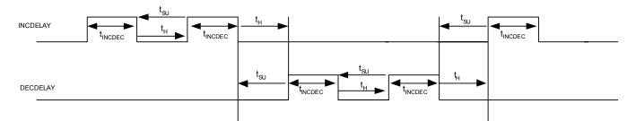
Figure 4. Output Phase Adjust Timing Diagrams (Pin Control)
