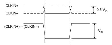
B. Operation with Differential Clock Input
