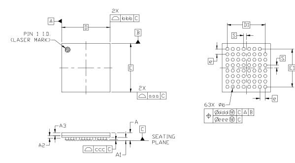
Figure 14. 63-Ball Plastic Ball Grid Array (PBGA)
