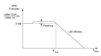
Figure 7. PLL Jitter Transfer Mask/Template
