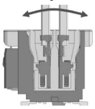
A structure that withstands stresses with deep mating. The thick external wall enhances strength against wall breakage. (fig.2)
