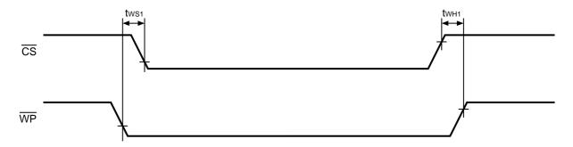
Figure 7 Valid Timing in Write Protect
