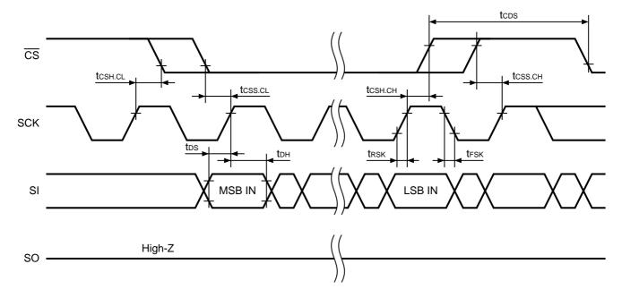
Figure 4 Serial Input Timing
