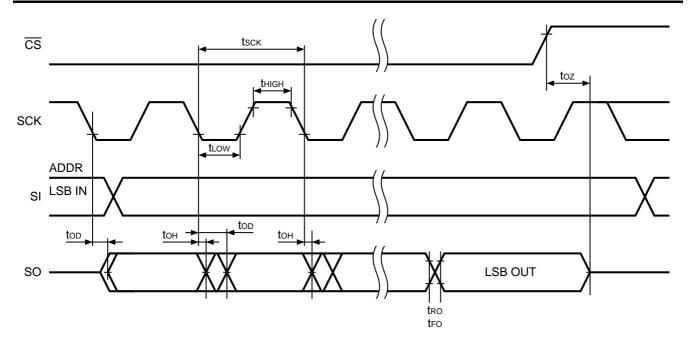
Figure 6 Serial Output Timing
