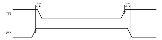
Figure 8 Invalid Timing in Write Protect
