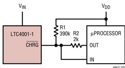
Figure 2. Microprocessor Interface
