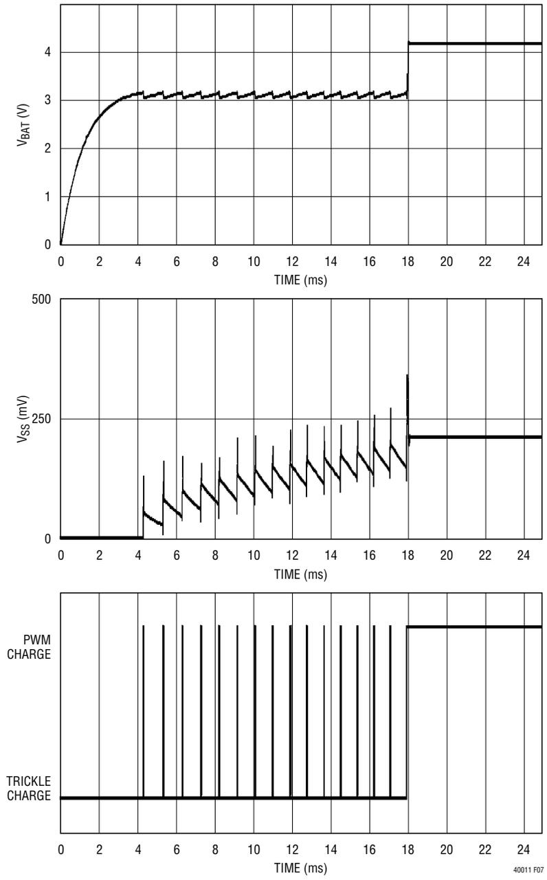
Figure 7. Battery-Less Start-Up
