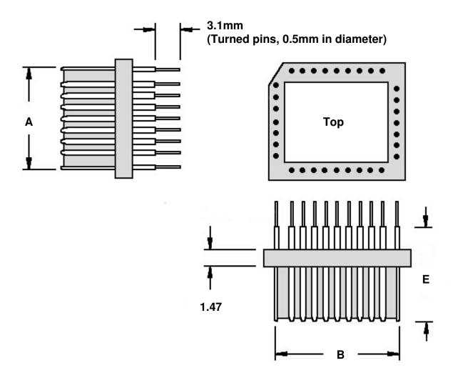
Number of pins shown is for illustration only. Plugs with longer pins may use two mouldings.
