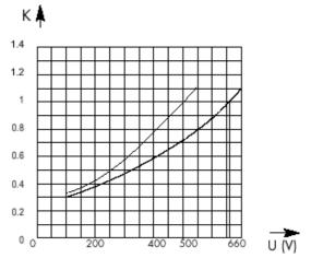
Mean curves show variation of total clearing time  $(I^2t_t)$  and total clearing duration  $T_t$  as a function of operating voltage U.
