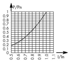
Curve enables computation of power losses P for a I<sub>N</sub>-rated fuse as a function of RMS current I (as a multiple of  $I_N$  for steady state operation).
