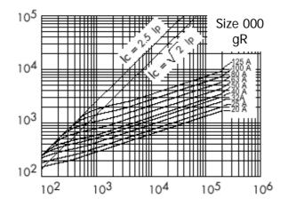
The curve below shows, for each rating, value of peak let-through current Ic as a function of available fault current Ip.
