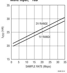
$I_{OVDD}$  vs Sample Rate, 5MHz Sine Wave Input, -1dB,  $O_{VDD}$  = 1.8V
