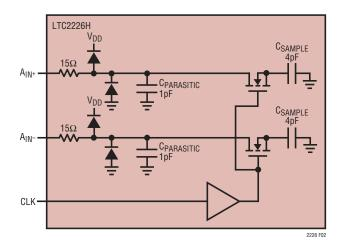
Figure 2. Equivalent Input Circuit
