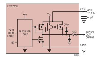
Figure 9. Digital Output Buffer
