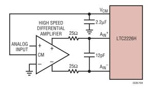
Figure 4. Differential Drive with an Amplifier
