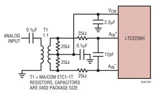
Figure 3. Single-Ended to Differential Conversion Using a Transformer
