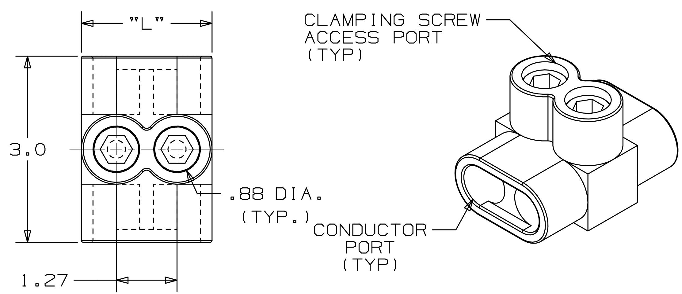
TWO PORT CONNECTOR BLOCK SHOWN WITH PLASTIC CLOSURE PLUGS REMOVED. SEE TABLE FOR DIMENSIONS OF PARTS WITH ADDITIONAL PORTS.
